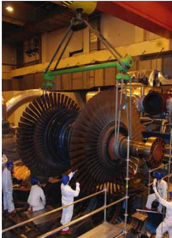
The removed rotor of a low-pressure turbine shows clear signs of corrosion from use.
