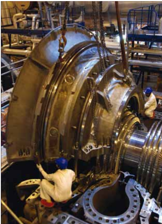
After servicing, the blade carrier casing is mounted back onto the low-pressure turbine.
